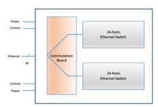
The unit can interface Ethernet via a large offering of space qualified connectors. Integrated filtering is designed to meet power input voltage, spikes, surges, transients and EMI/EMC requirements of typical deployments (including Deep Space Gateway). The TSU enables deterministic Local Area Network (LAN) switching and time synchronization across extended operating temperature ranges, shock/vibration radiation and conditions.
