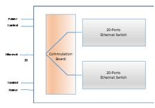
The unit can interface Ethernet via RJ45 type connectors or high performance circular connectors. Integrated filtering is designed to meet power input voltage, spikes, surges, transients and EMI/EMC requirements of typical space deployments. The REG enables reliable Local Area Network (LAN) switching across extended operating temperature ranges (-23°C to +63°C), shock/vibration and radiation conditions.
