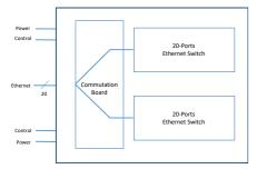
The unit can interface Ethernet via RJ45 type connectors or high performance circular connectors. Integrated filtering is designed to meet power input voltage, spikes, surges, transients and EMI/EMC requirements of typical space deployments. The REG enables reliable Local Area Network (LAN) switching across extended operating temperature ranges (-23°C to +63°C), shock/vibration and radiation conditions.
